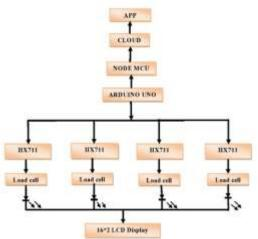
Figure 1:Block Diagram of Proposed Model
